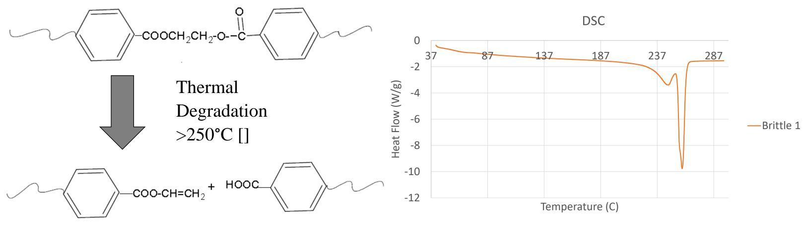
recycling PET are due to its thermal degradation
