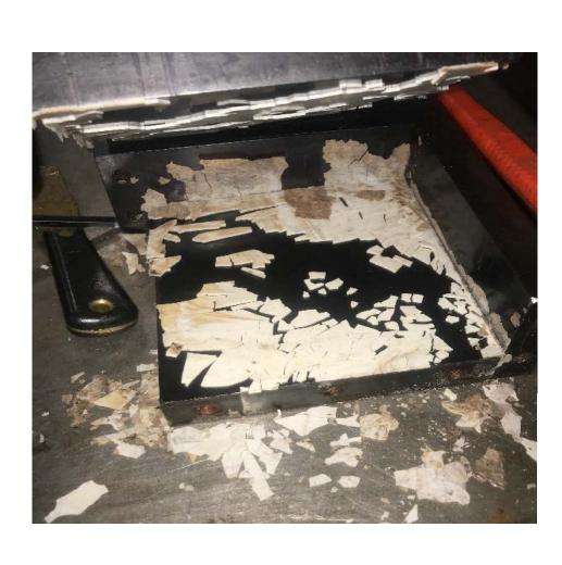
Figure 4: Compression molding; 2 hour heating time; 257°C; 1 MPa; Obvious thermal degradation
